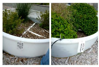
Soil Column Tank with plantings of slough sedge, red osier dogwood, and red switch grass and tank showing label of 60% sand and 40% compost.
