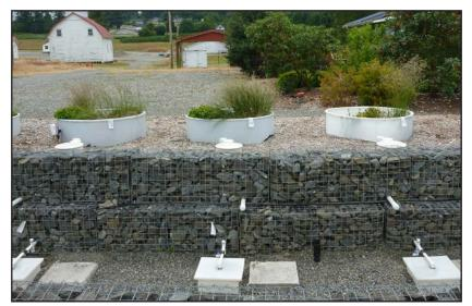
Soil tank columns and collection of water after treatment.
