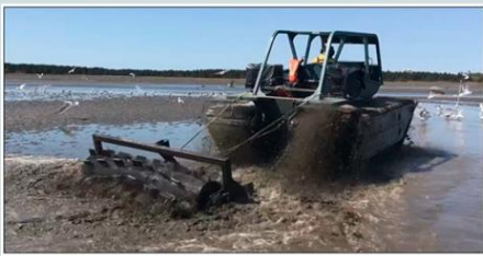
Figure 2. WDNR Marshmaster-2LX towing the roller - chopper "dry harrow" implement at Grassy Island, treating a dry harrow plot.
