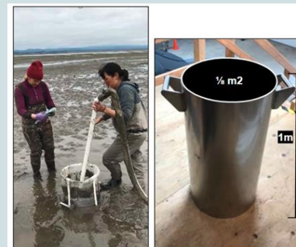
Figures 4 and 5. Large core hydraulically pumped out and used for assessing shrimp density. The core is one meter deep with a surface area of 1/8 m 2 .
