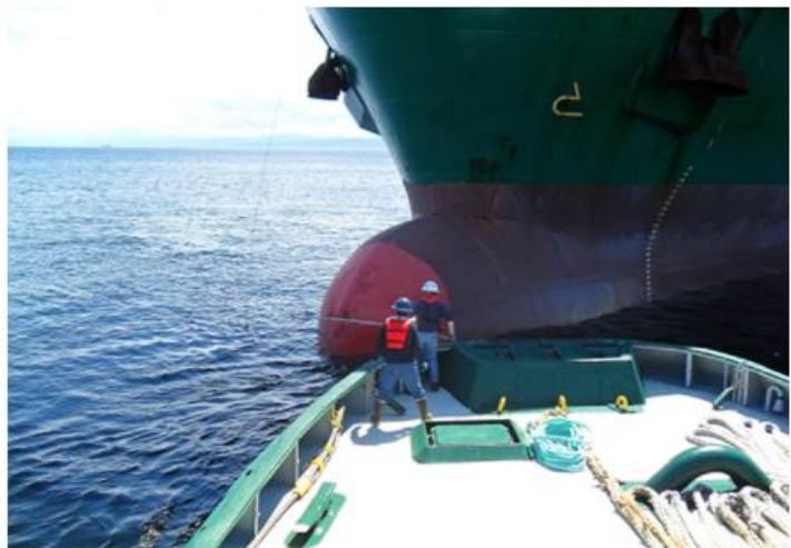
Workers aboard the Jeffrey Foss, one of several vessels contracted over the years to fill the 24/7 role of the Neah Bay tug, connect a tow line to a stalled ship. (Washington State Department of Ecology photo)
