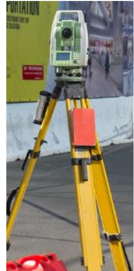
Figure 2 | A theodolite measures angles, distances, elevation, and more to calculate distances of objects from one another. Image by Billie Grace Ward, Flickr CC 2.0
